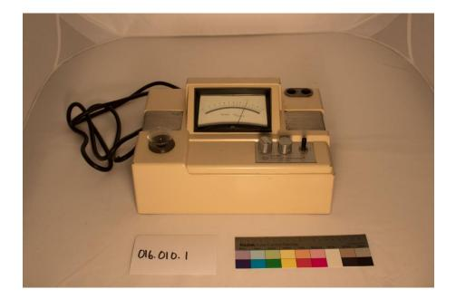
This hemophotometer is a tan, metal machine with an electrical cord. On the back, there is a fuse knob and outlet for another plug. On the top, there is a gauge with a needle indicating grams Hb/100 ml. The gauge is marked from 4 to 20. There is an opening with a plastic funnel inside a rubber ring on the proper right. Two dials and a switch are located on the proper left bottom, and two openings in rubber on the proper left top. Both sides have metal vents on the center top of the machine.
